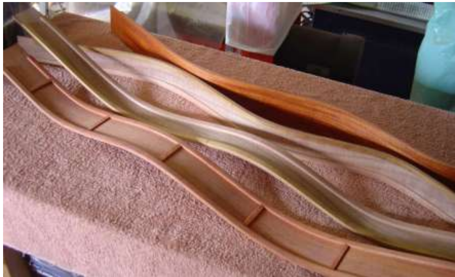
Figure 12.8. Sides with side linings attached
