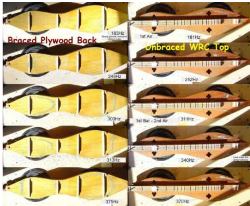
Figure 6.7. Ply back, braced; WRC top, no braces
