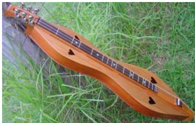
Figure 5.10. Dulcimer #56 (same as #57) – three arches, grooved Kauri Pine top.
