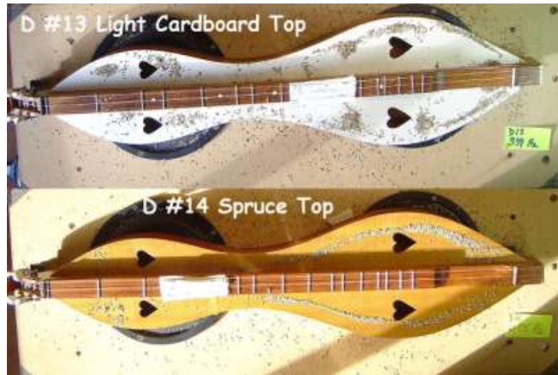
Figure 1.7. A vibration mode for manila folder and spruce dulcimer top
