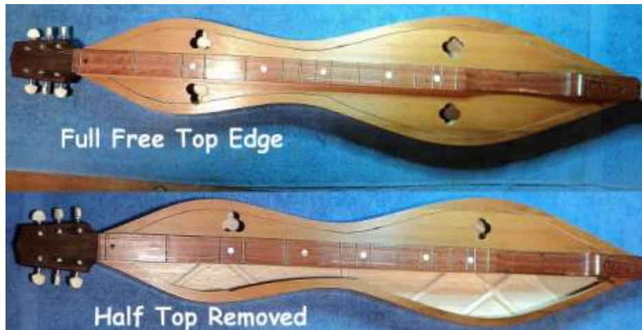
Figure 13.18. Test dulcimer with free top edge, then half top removed
