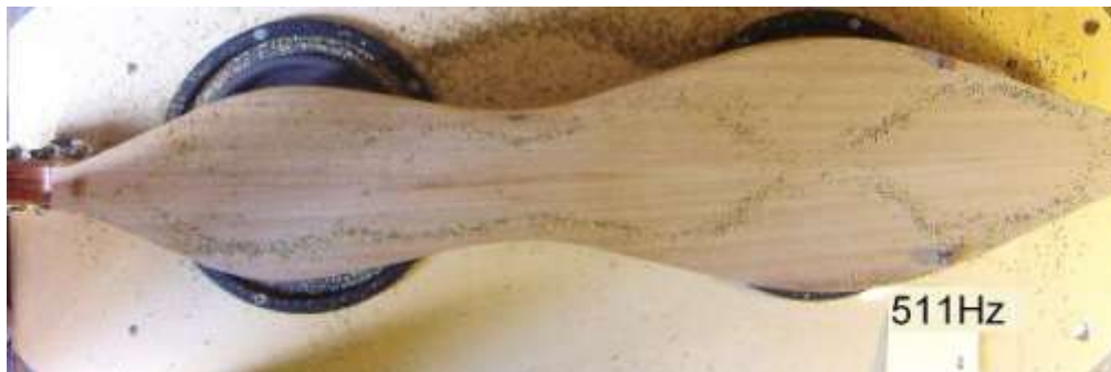
Figure 7.6. Vibration pattern for 3.5 inch waist
