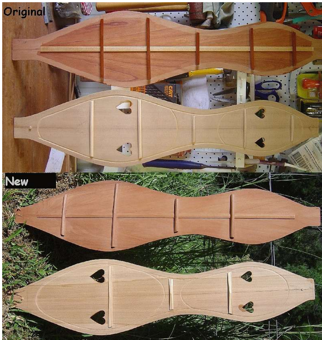
Figure 5.12. Bracing in original and new dulcimer tops
