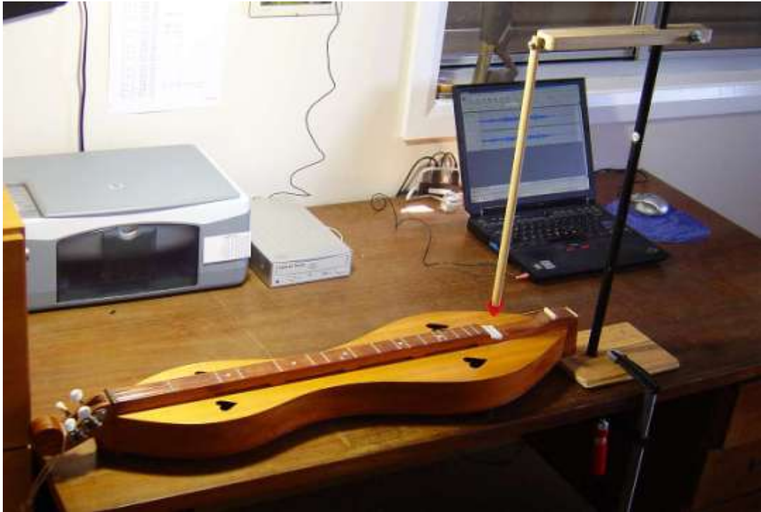
Figure 1.1. Dulcimer #13 – Pendulum String Striker
