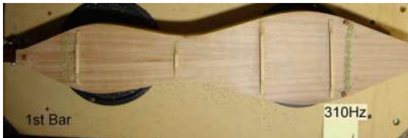
Figure 6.2. Unbraced WRC top; externally braced Stringybark back
