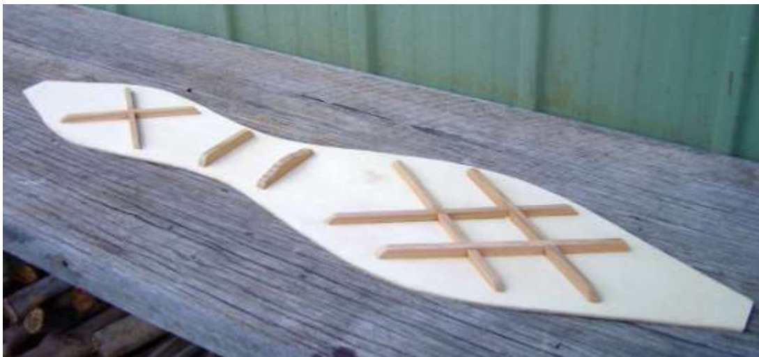
Figure 13.5. Hoop pine plywood back
