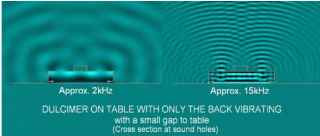
Figure 14.12. Simulation of sound radiating from the dulcimer back/table gap
