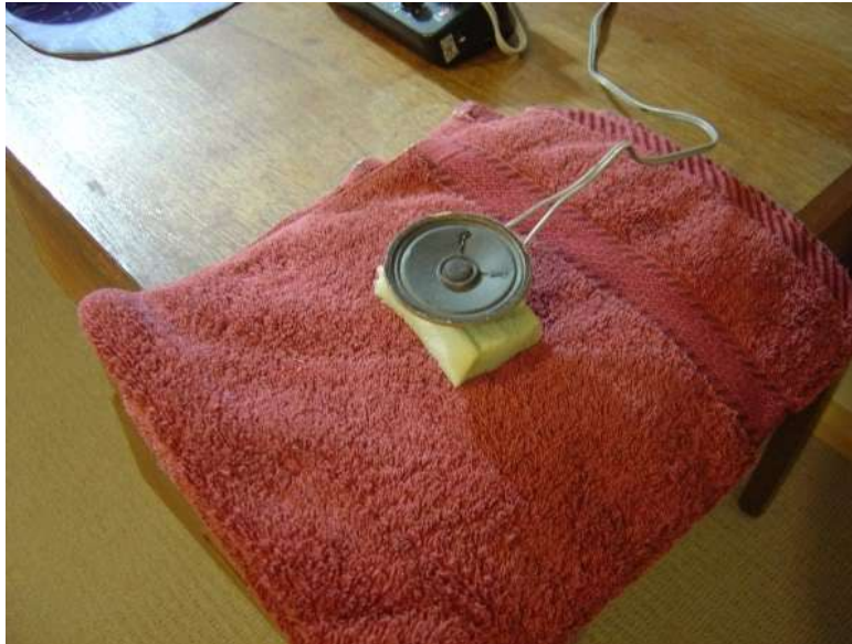
Figure 2.3. Speaker on foam pad
