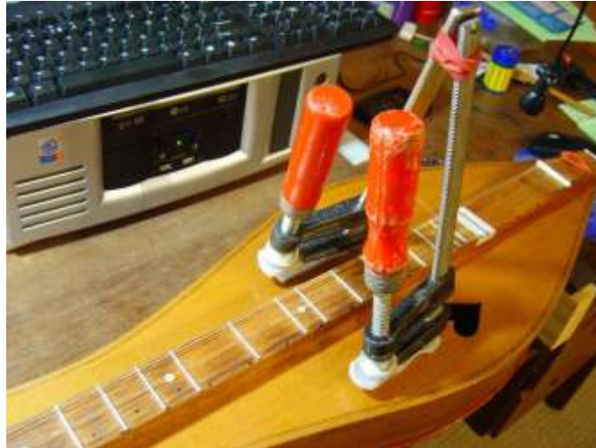
Figure 16.4C. 544g top plate weight added
