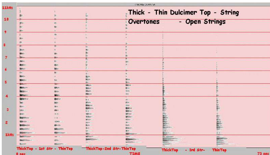
Figure 4.15. Spectrogram comparison for thick and thin topped dulcimers
