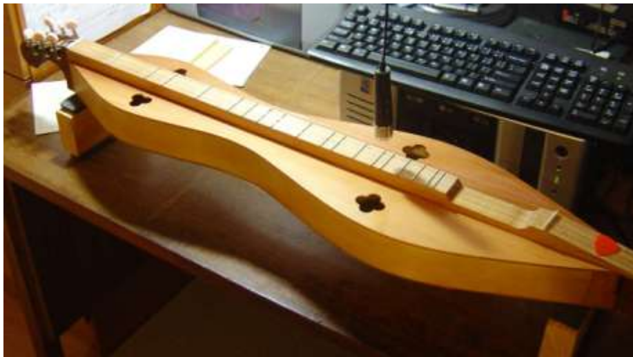
Figure 8.6. Test dulcimer with original fretboard with low arches
