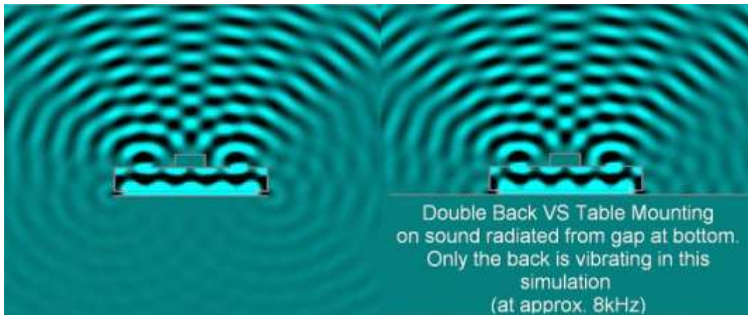
Figure 14.13. Simulation of sound radiating from the inner back of a double backed dulcimer and from the back of a single backed dulcimer with feet played on a table.
