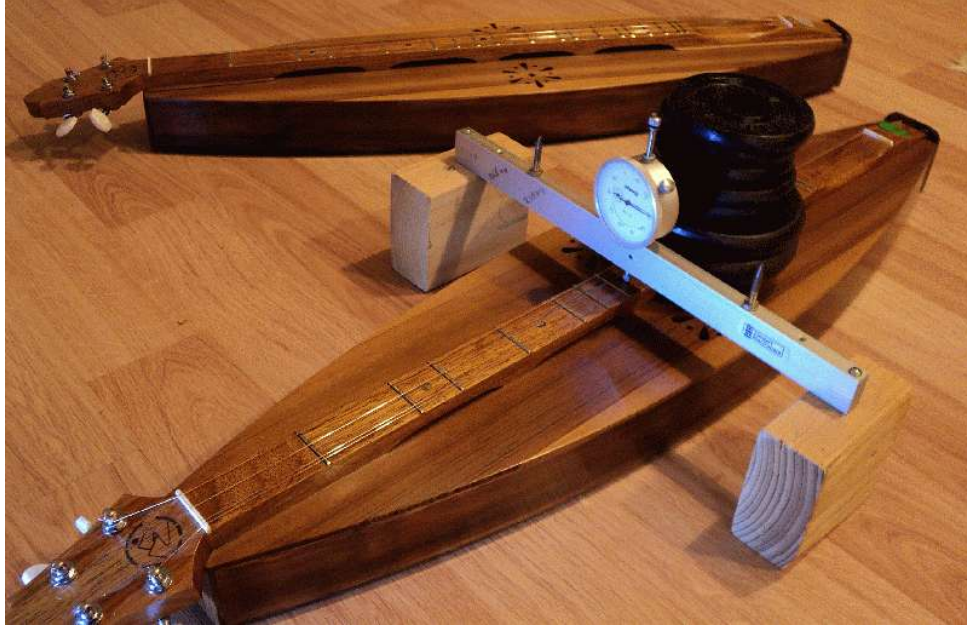
Figure 4.19. Dulcimer suspended on small feet — top/body deflection
