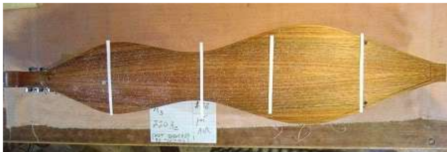
Figure 3.7. Dulcimer No. 38 vibration pattern
