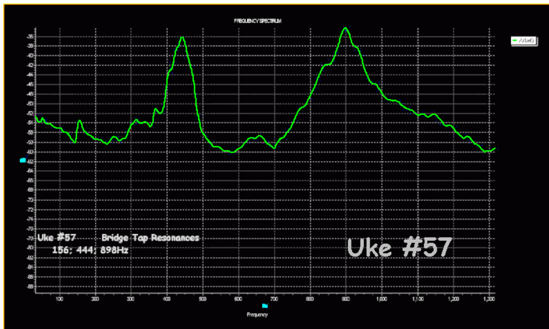
Figure 3.21. Resonance spectrum for Uke#57
