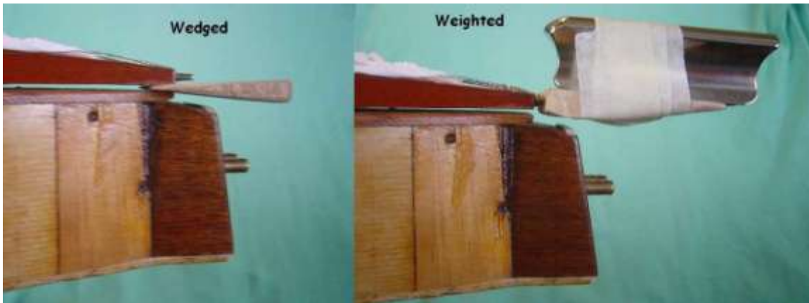
Figure 10.13. Wedged and weighted fretboard end
