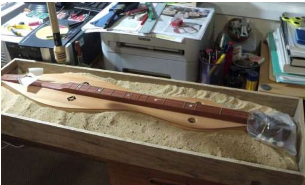
Figure 11.30. Dulcimer buried in sand to immobilize back and sides
