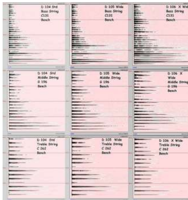
Figure 14.6. Sound spectrograms for individual strings
