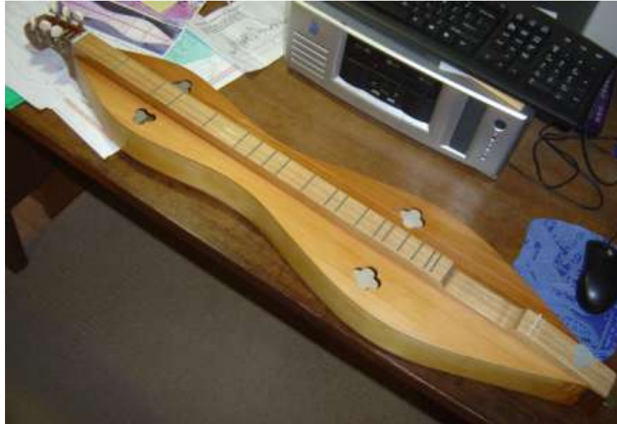
Figure 7.9. Test dulcimer with western red cedar top and 2mm high arches
