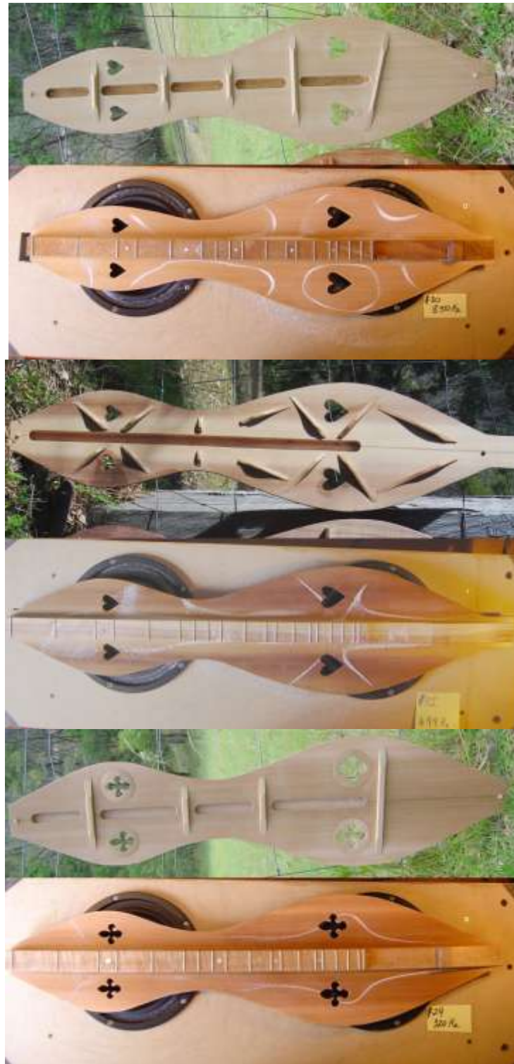
Figure 3.3. Examples of vibration patterns for braced dulcimer tops
