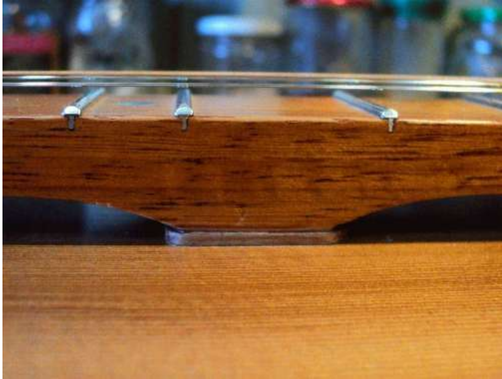
Figure 4.14. Thin-topped dulcimer after fretboard pads added.
