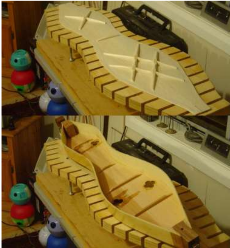
Figure 11.6. Western Red Cedar top and Balsa back bracing
