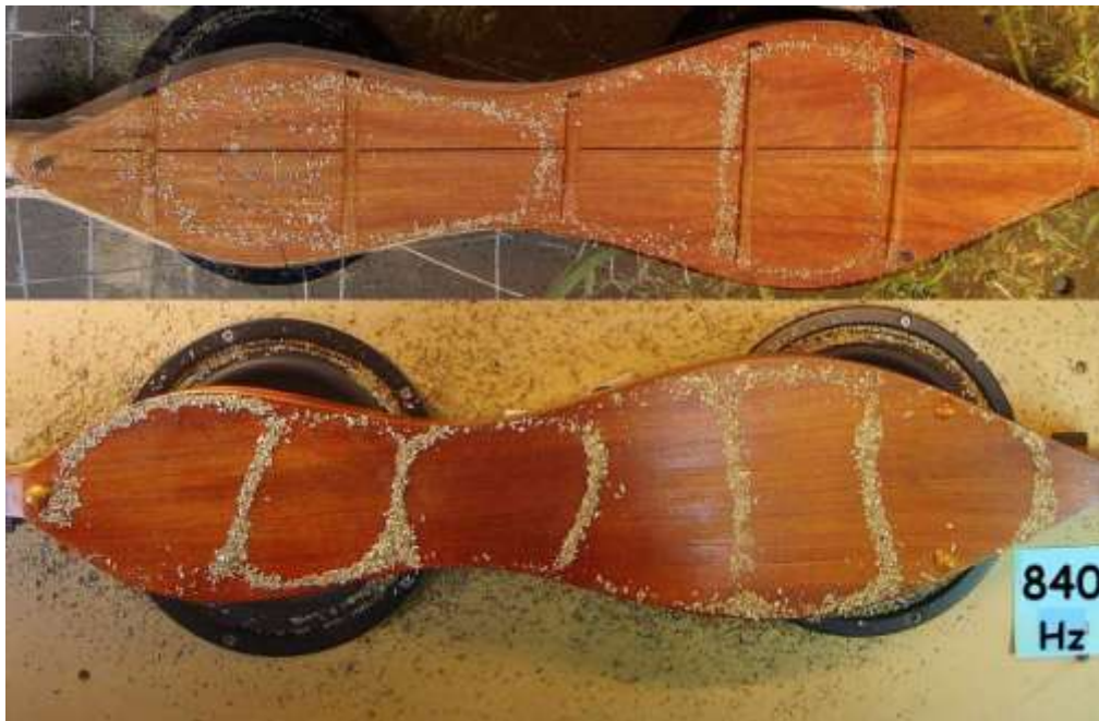
Figure 11.27. Similar back vibration pattern for braced (upper panel) and unbraced back (lower panel).
