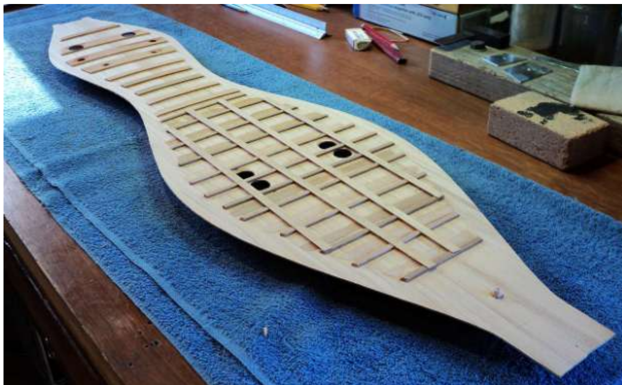
Figure 11.34. #127 Kauri Pine 1.6mm lattice braced top
