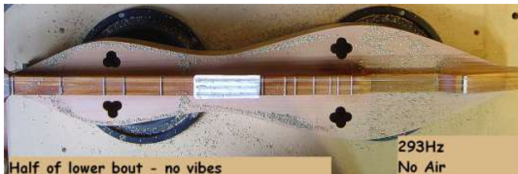
Figure 9.12. A vibration mode for the full arched fretboard where the lower bout stopped vibrating.
