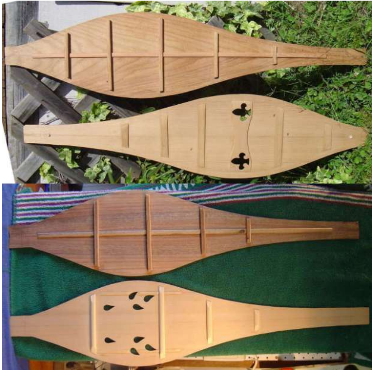
Figure 11.16. Teardrop dulcimer bracing
