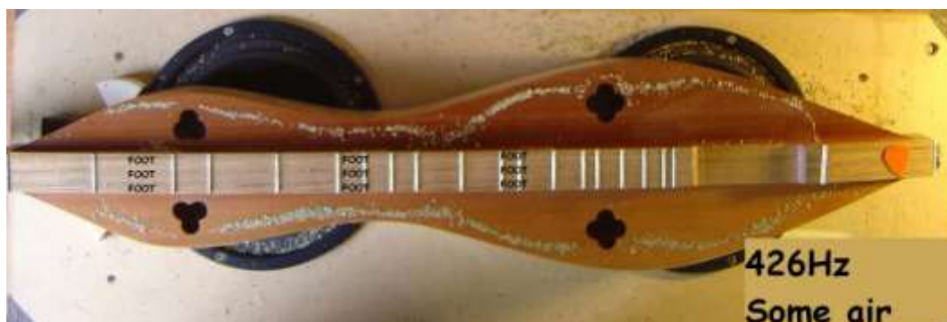
Figure 11.10 Vibration pattern avoiding feet
