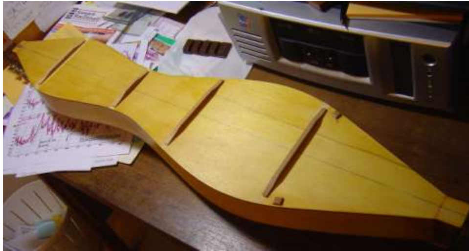
Figure 11.1. Back braces installed on outside of the test dulcimer
