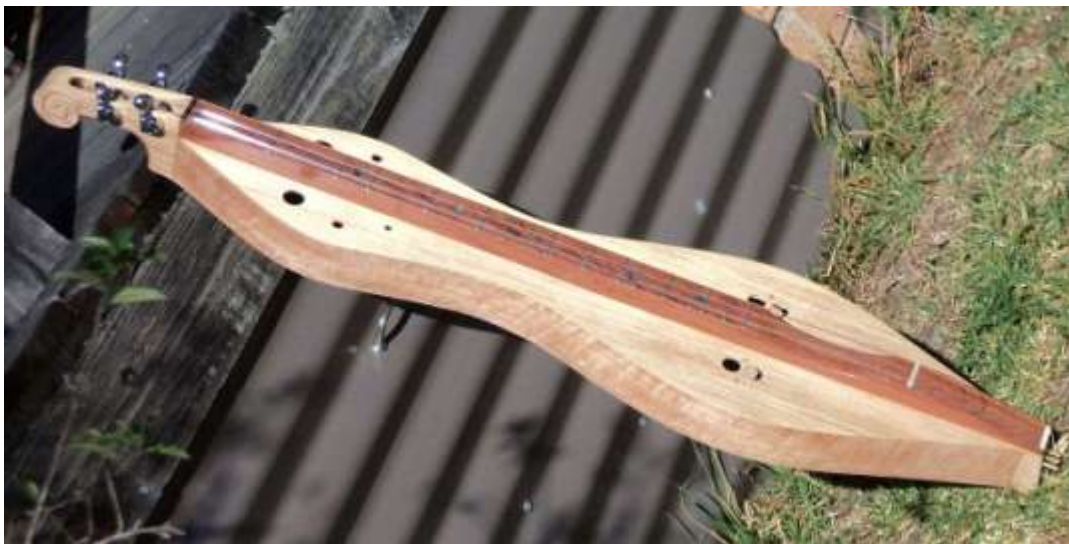
Figure 11.35. #127 Thin sided, lattice-braced, Balsa-core fretboard Yellow Stringybark dulcimer
