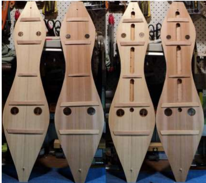
Figure 8.13. Two Dulcimer Tops with fretboard channels closed then opened.
