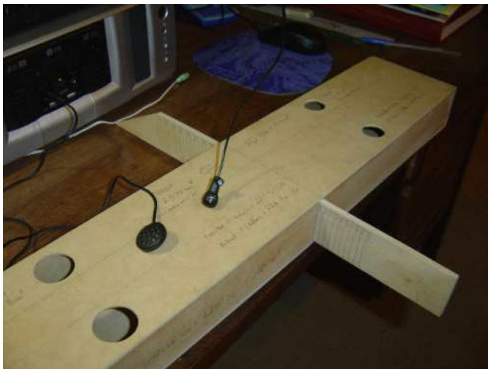
Figure 7.4. Box set up to measure waist effects
