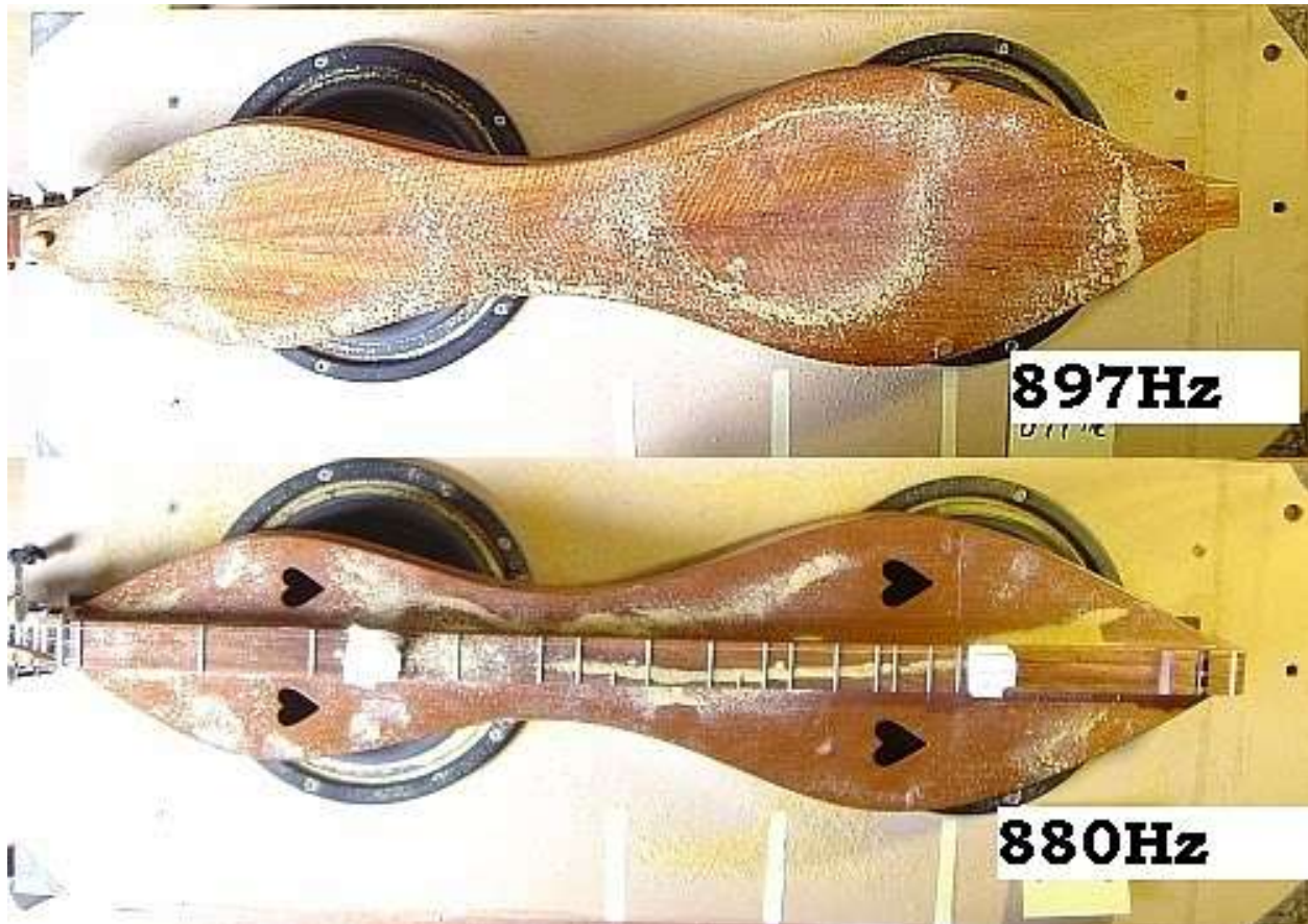
Figure 2.11. Evidence of twisting vibration
