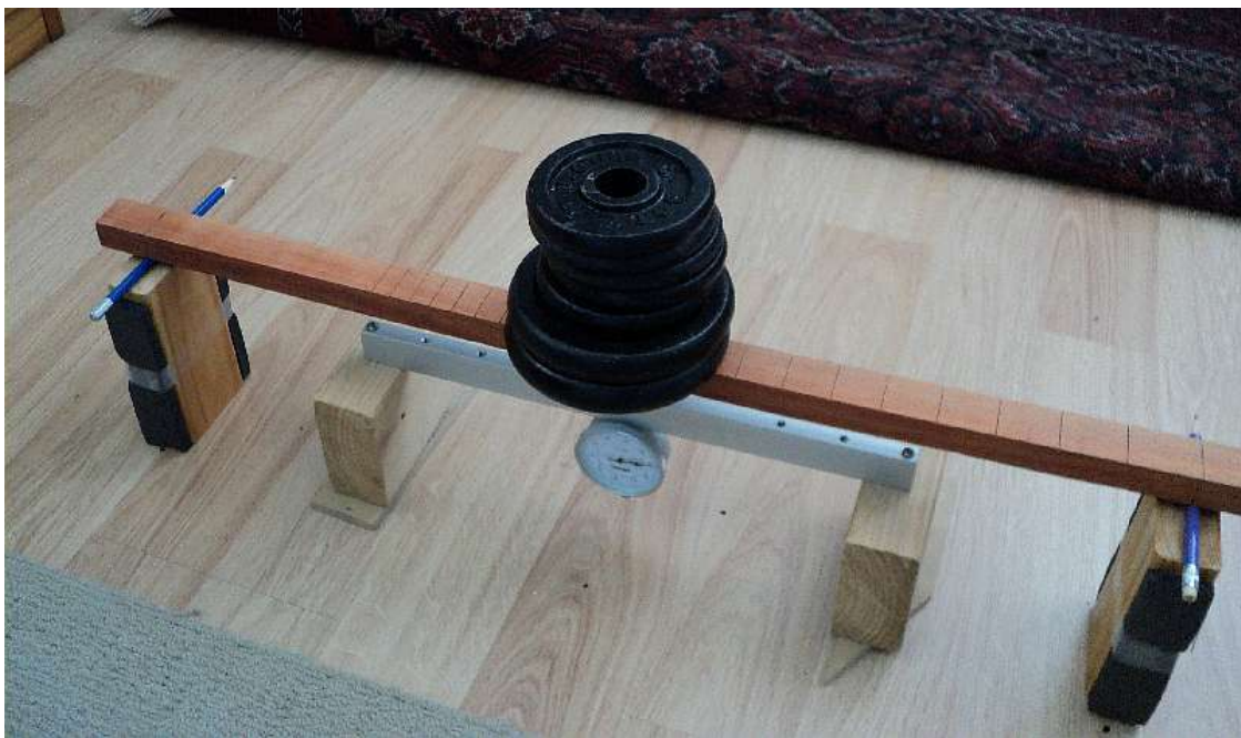
Figure 7.17. Fretboard deflection measurement with fret cuts
