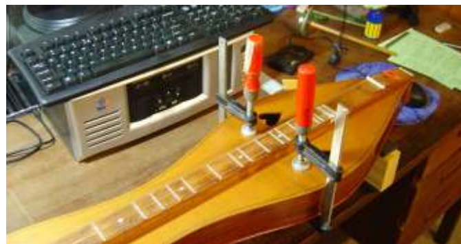
Figure 16.4D. 544gm top/back clamp
