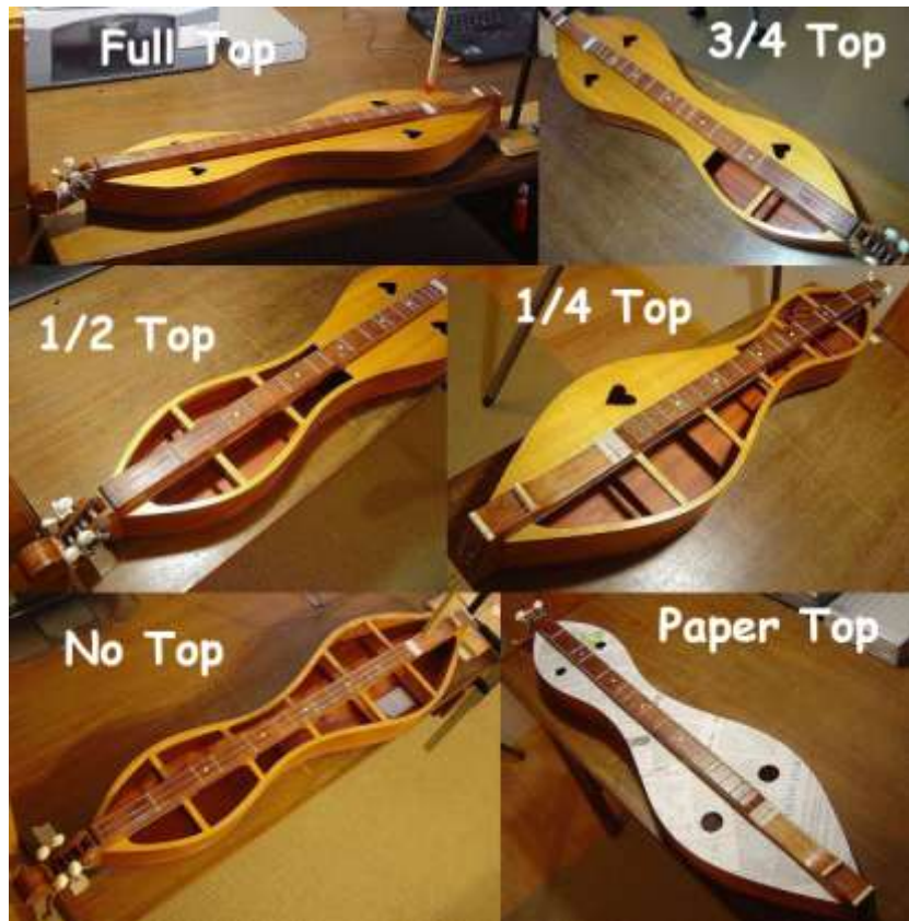
Figure 1.2. Dulcimer #13 - Stages of top removal
