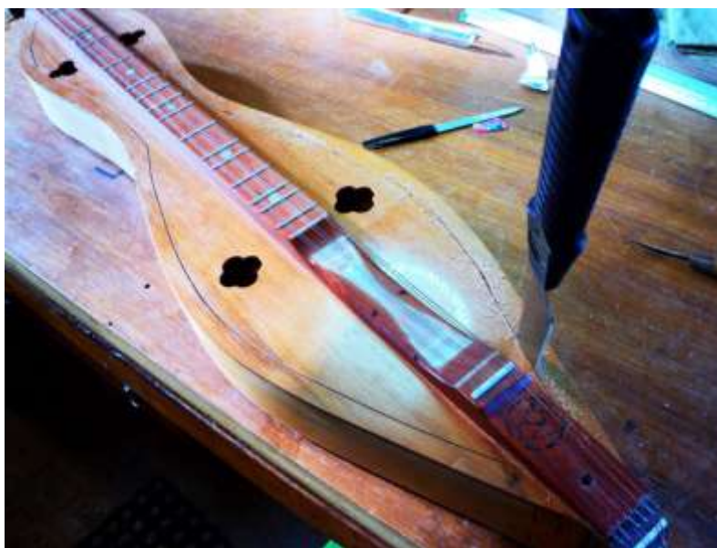
Figure 13.17. Cutting the top edge of the test dulcimer
