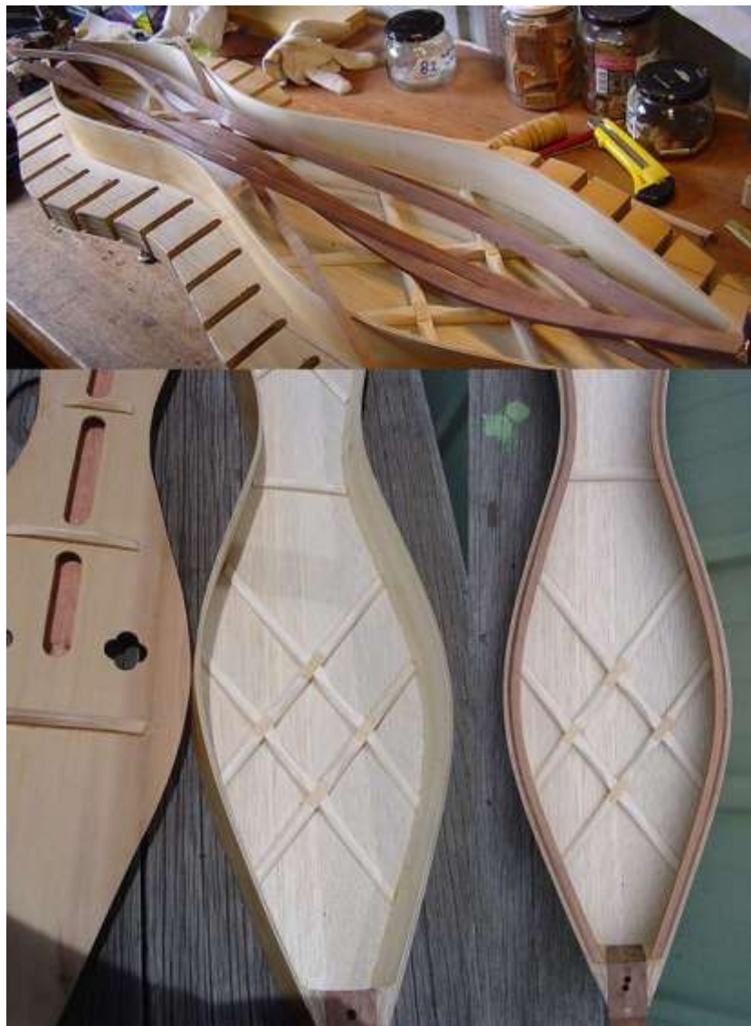
Figure 12.3. Test dulcimer before and after installation of extra wide and dense side linings
