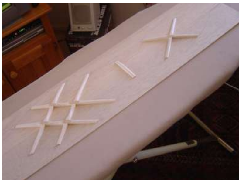
Figure 11.5. New Balsawood back and bracing
