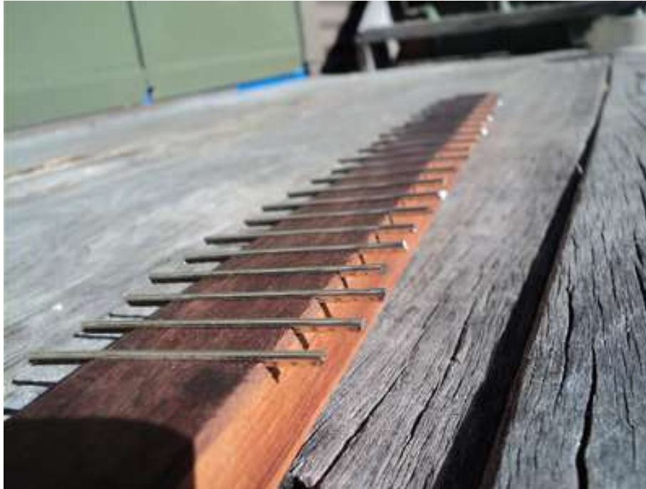
Figure 7.18. Fretboard with frets added
