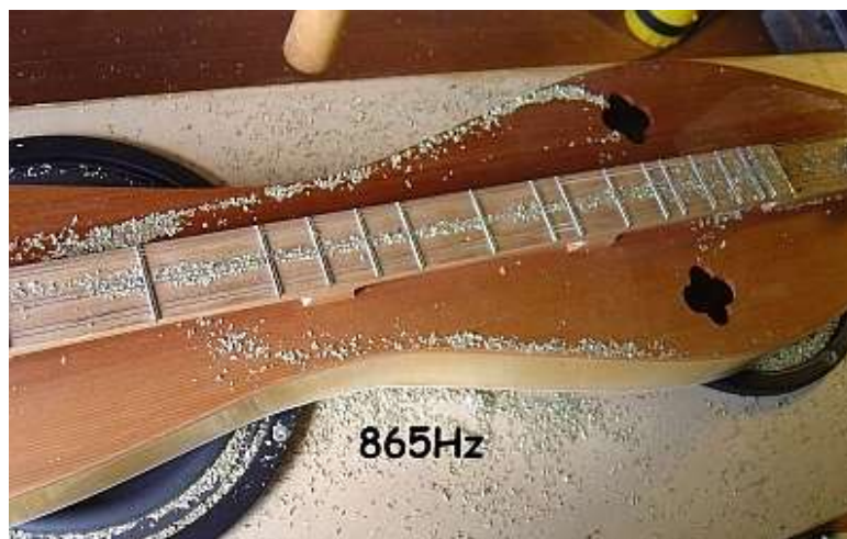
Figure 11.14. Twisting vibration mode
