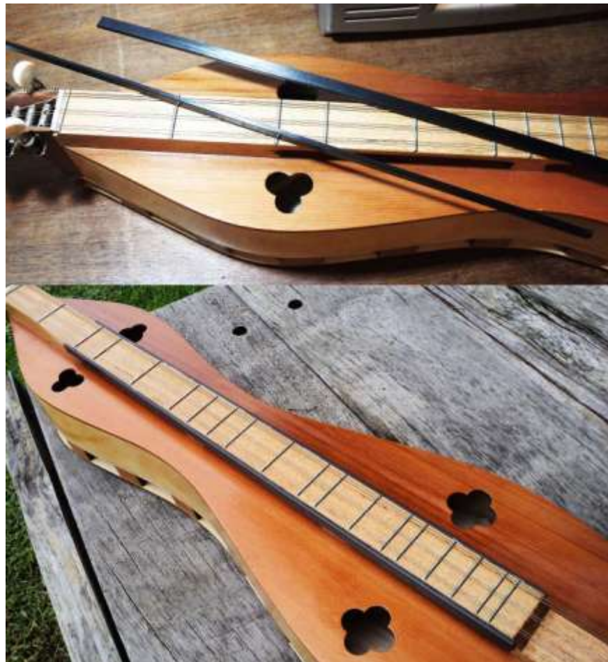
Figure 7.11. Test dulcimer with carbon fiber bars
