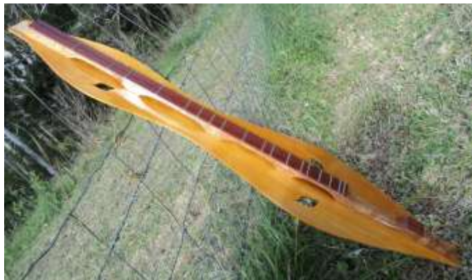
Figure 11.19. Top with fretboard
