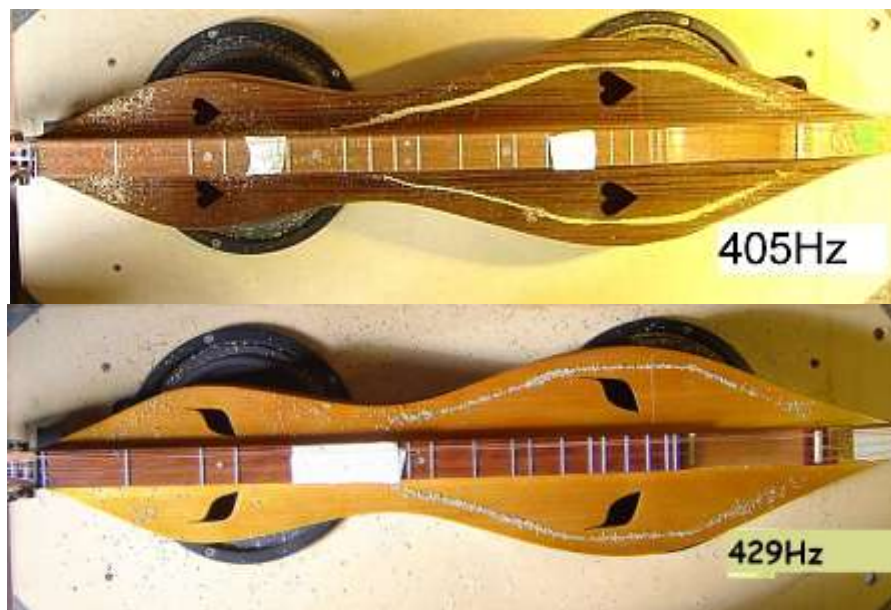
Figure 11.12. Vibration pattern for continuous fretboards
