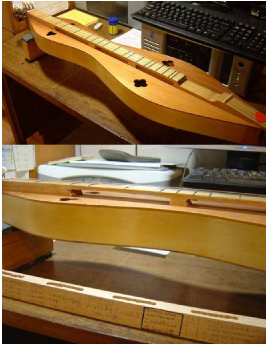
Figure 8.7. Test dulcimer with fretboard modified to make arches higher.
