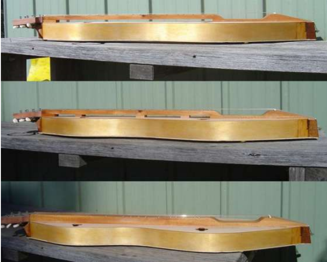
Figure 9.6. Three test fretboards - full arch, four arches and hollow
