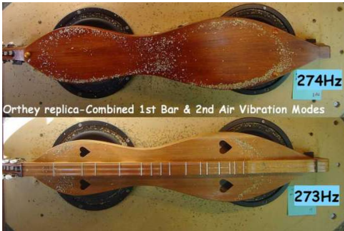
Figure 11.24. Vibration pattern in Orthey replica
