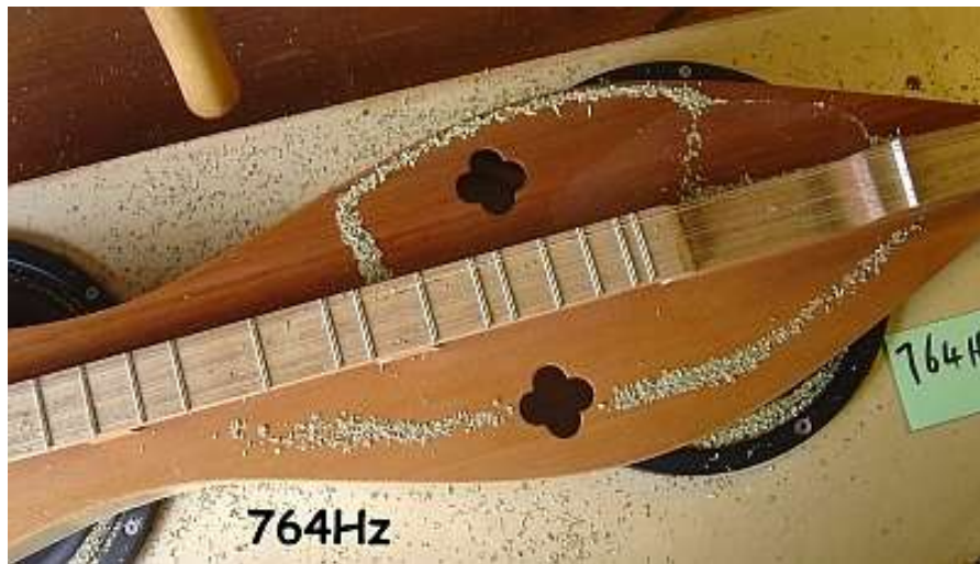
Figure 11.13. Asymmetrical vibration pattern
