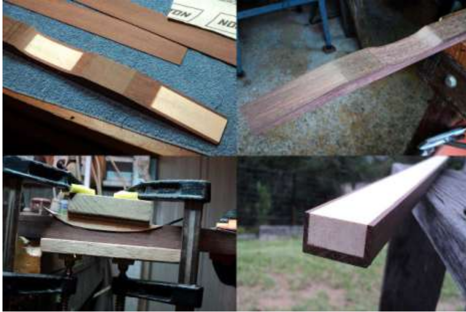
Figure 11.32. Balsa core fretboard construction
