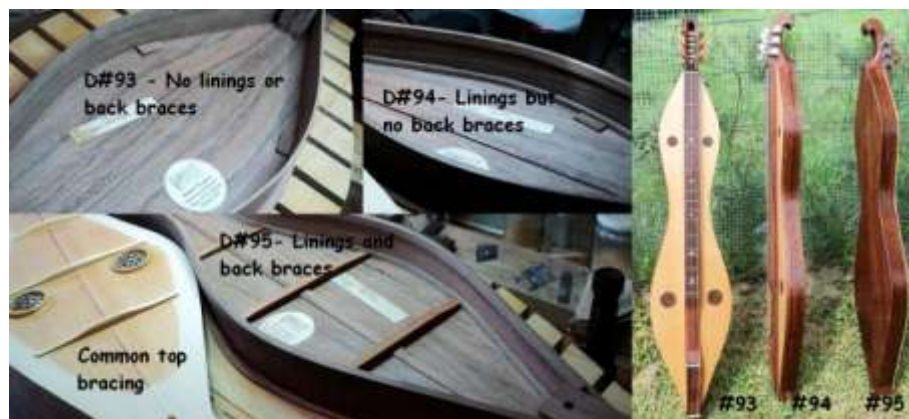
Figure 12.9. Three dulcimers with different linings and back bracing
