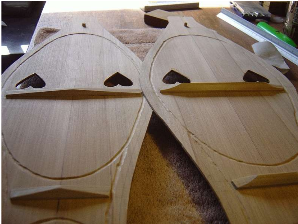
Figure 5.13. Bracing pattern in two new dulcimers
