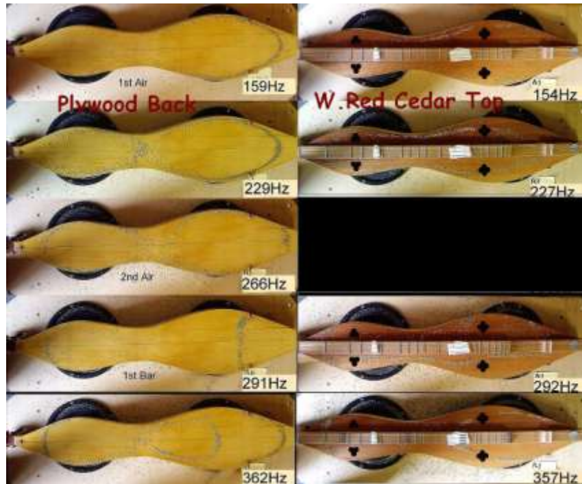
Figure 6.5. Ply back, no braces; WRC top, no braces.
