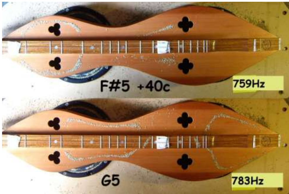
Figure 9.7. Two top resonances close in frequency with quite different vibration modes
