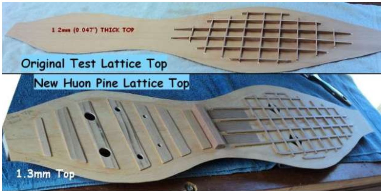
Figure 11.31. Test dulcimer with lattice bracing
