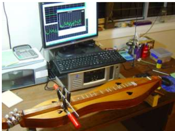
Figure 16.4B. 544gm fretboard weight added.
