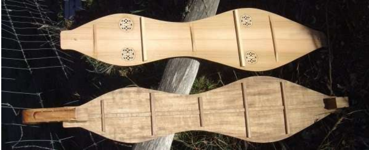
Figure 8.1. Dulcimer bracing pattern
